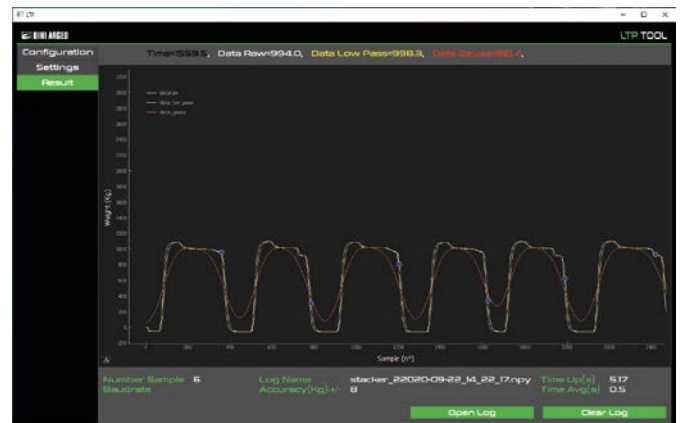
LTP TOOL: Software for weighing system configuration.
