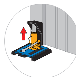
SOLUTION 2 Weigh the container by lifting it, using the jacks standing on the platforms.
